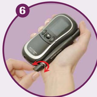
**6** Twist the cap to the desired depth setting (11 settings in total).
