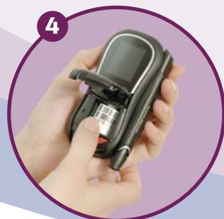
4 Insert new test strip drum.
