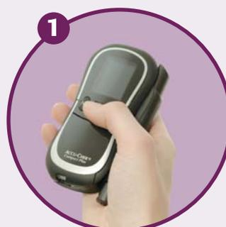
1 Pull down the test button to advance a test strip.
