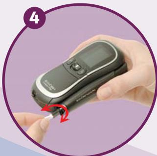
**4** Remove the protective cap from the lancet with a twisting motion.
