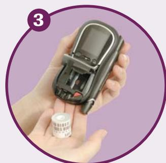
3 Tip the meter forwards, the test strip drum drops out.
