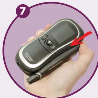
**7** Press the plunger all the way down. The plunger returns about a third of the way. The lancing device is now primed.
