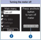
Select 2 (press and release the  $\textcircled{\basis}$  button) selects the highlighted *Turn off* command  $((\fbox))$ .
