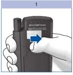
Push the slide button for the finger pricker in the direction of the arrow as far as it will go. Hold the slide button in that position.
