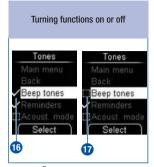
A tick 🗸 🚯 in front of an option means that the function is on.
