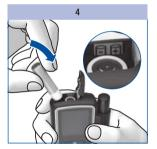
Insert two new batteries in the battery compartment. Ensure that the polarity (-+ and --) of the batteries is correct.
