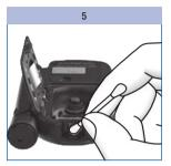
Carefully dab the measuring optics and the front opening of the meter with a slightly dampened cotton swab.
