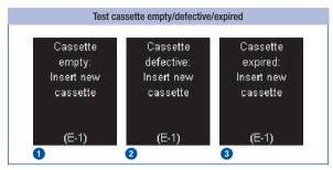
If the test cassette in the meter is empty  $\bigcirc$  or defective 0 or has expired 0, the appropriate message appears after the display check and the number of available tests (see also page 120). Shortly after this, the meter turns off automatically.
