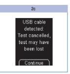
If you connect the meter to a PC while a test is in progress, the test is cancelled and a message appears on the screen.
