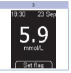
Testing is complete after approx. 5 seconds, depending on the blood glucose concentration. The test result appears on the screen and the beep tone sounds. The meter saves the test result at the same time. The used test area is transported away from the tip of the cassette.
