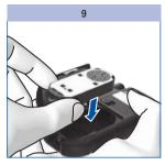
Re-insert the test cassette in the meter.
