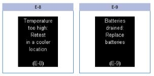
Move to a place where the temperature is at most +40 °C and wait for the temperature of the meter to adjust to this temperature.
