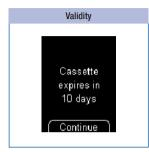
This message appears at the start of a test if the test cassette is only valid for 10 more days. The message is repeated when the test cassette is only valid for 5, 2 and 1 more day(s).
