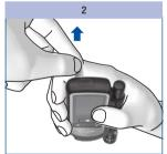
Pull the protective strip of the batteries backwards out of the meter.
