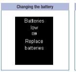
This message appears when the batteries are almost empty. It appears every time you turn the meter off if you have not yet changed the batteries. After the message appears for the first time, you can still perform about 50 tests.
