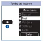
Pressing and holding the button (for approx. 2 seconds) turns the meter on. After the display check, the meter first displays the number of tests still available on the test cassette and then opens the main menu.
