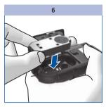
Insert the new test cassette in the meter with the silver side facing upwards.
