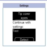
This message appears if you are in the process of changing a setting (for example, the date) or entering a setting again (for example, a reminder) and open the tip cover.
