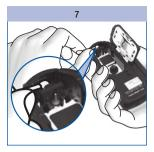
Carefully dab the interior of the tip cover with a slightly dampened cotton swab.
