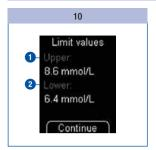
The meter displays the upper **1** and lower **2** limits of the concentration range. The concentration range displayed depends on the colour of control solution selected.
