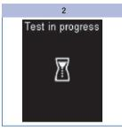
Remove your finger from the test area when the beep tone sounds and *Test in progress* is displayed.
