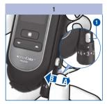
Push the lever ① in direction A and then back again in direction B.
