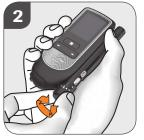
Rotate the cap, until the marking shows thedesired penetration depth. Start with a medium penetration depth, i.e. 3.
