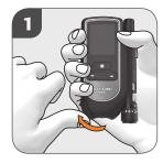
Open the tip protector to the stop. Only then can you open the cartridge compartment and insert the test cartridge.
