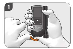
**Opening** Open the tip protector. The measuring device switches on.
