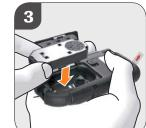
Insert a new test cartridge into the measuring device. Close the lid of the cartridge compartment and the tip protector.
