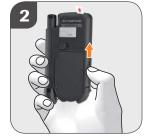
Push the locking button of the cartridge compartment lid upwards.
